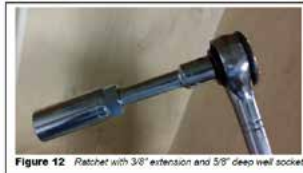
Figure 12 Ratchet with 3/8" extension and 5/8" deep well socket
