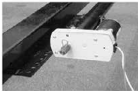
Fig. 3 - Hex Head Crank Extension
