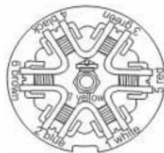
7-way trailer plug car end, rear view
