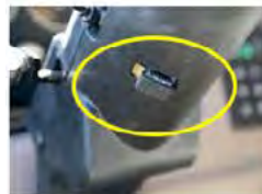
Hazard Warning Flasher
