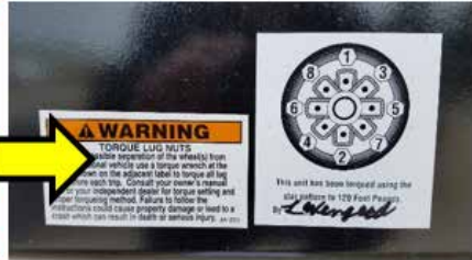
Lug nut torque pattern and warning label
