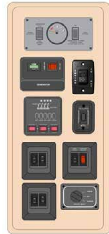
Command Center Panel w/Switch Modules
