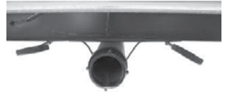
Black/Grey Tank Drain and Valves
