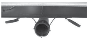
Black/Grey Tank Drain and Valves
