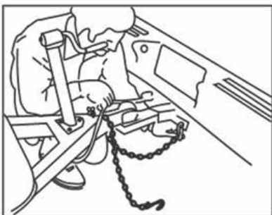
2. Criss-cross left chain and attach to right mounting slot in tow vehicle hitch.
