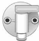
Exterior Fresh Water Drain
