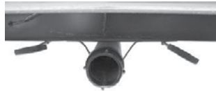
Black/Grey Tank Drain and Valves
