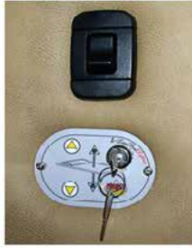
Fig.2 Key OFF (Vertical)
