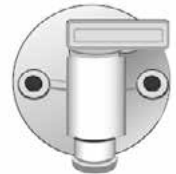
Exterior Fresh Water Drain
