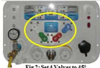
Fig 2: Set 4 Valves to 45°
