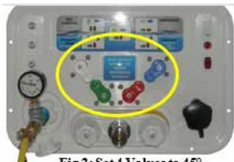
Fig 2: Set 4 Valves to 45°
