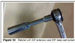
Figure 12 Ratchet with 3" extension and 5/8" deep well socket
