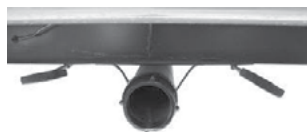
Black/Grey Tank Drain and Valves
