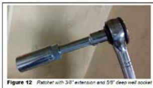
Figure 12 Ratchet with 3" extension and 5/8" deep well socket
