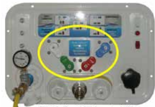
Fig 2: Set 4 Valves to 45°
