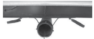
Black/Grey Tank Drain and Valves
