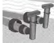
Low Point Drains
