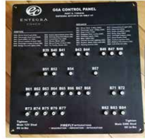
GFCI Breaker Panel
