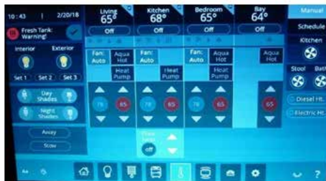
Example touch screen system climate controls
