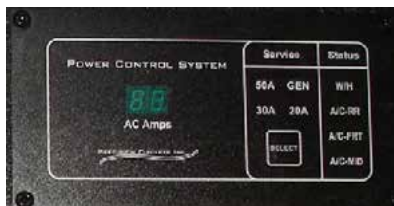
50A System Panel
