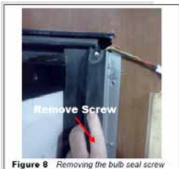
Figure 8 Removing the bulb seal screw
