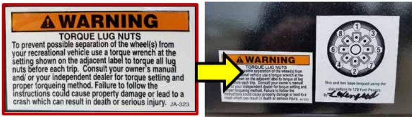
Lug nut torque pattern and warning label
