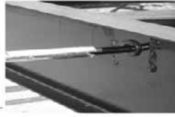
Fig. 2 - Through Frame Crank Extension w/Pin
