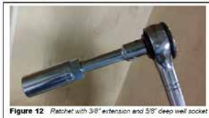
Figure 12 Ratchet with 3/8" extension and 5/8" deep well socket
