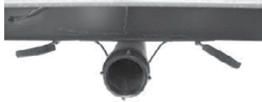
Black/Grey Tank Drain and Valves
