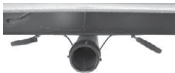
Black/Grey Tank Drain and Valves
