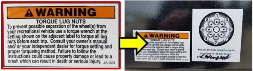
Lug nut torque pattern and warning label
